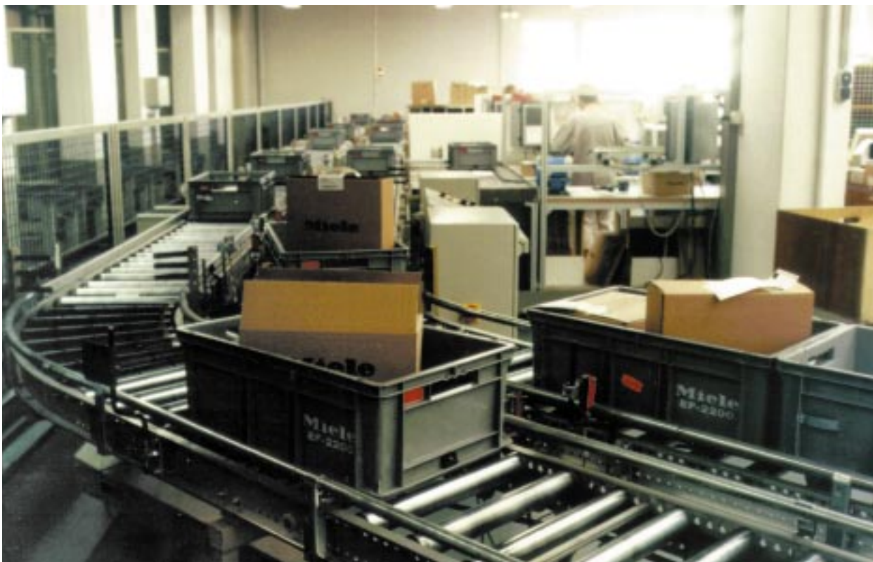
Spare parts order picking sped up with tagged box system.
