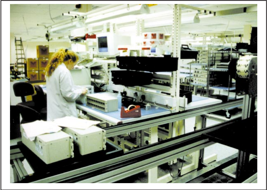
Box-build assembly process made easier by tagging conveyor pallets.
