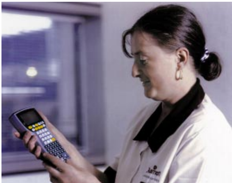
Supervisor reads transponder at specific location to get display of requested tasks.
