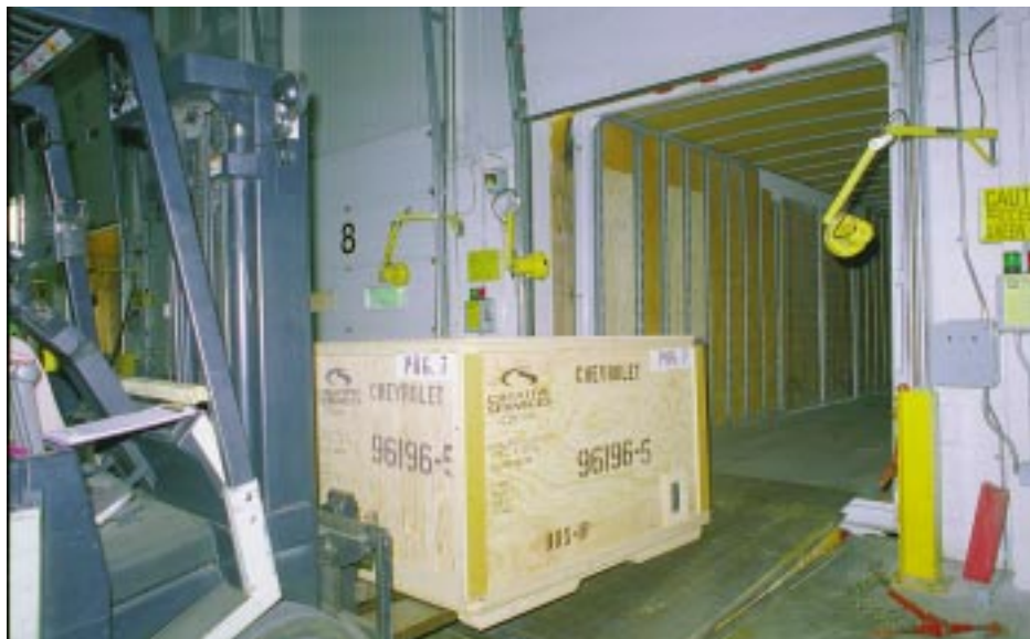
Tagged crate automatically triggers "green light" to allow loading shipment.
